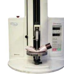
Reference Upper jig 20 mm dia. Part No.346-51687-10 Lower jig Part No.346-51687-12
