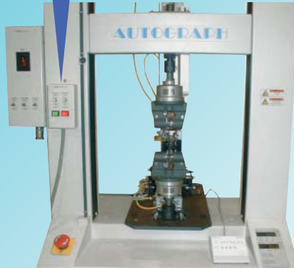
System example with AGS-J + automatic SES + pneumatic grips
