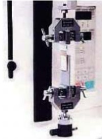
Tensile testing jig set Part No.346-51690-03
