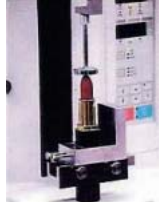
Upper jig Compressive elasticity Part No.346-51687-08 Lower jig Lipstick test jig Part No.346-52022 Bending centers for JIS bending tests Part No.346-51687-08
