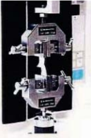
Compact, flat grips for tensile testing Part No.346-51690-03
