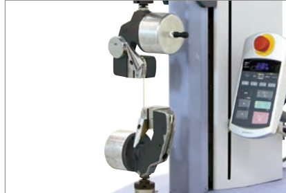
• 1 kN pneumatic capstan type grips for yarn Ⓢ Adapter for AGS series jig \phi 16
