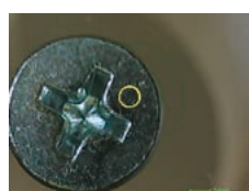
Top of Screw (Measurement at 1 mm dia.)
