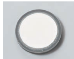
Press form the powder with a press machine (briquette press method).
