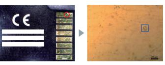
Observation image of the foreign matter on the terminal by 15× Cassegrain objective mirror.
