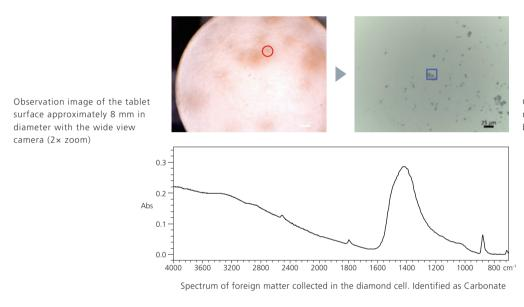
Observation image of the foreign matter on the diamond cell by 15× Cassegrain objective mirror.
