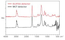
The infrared spectra of polyvinyl chloride (PVC)
